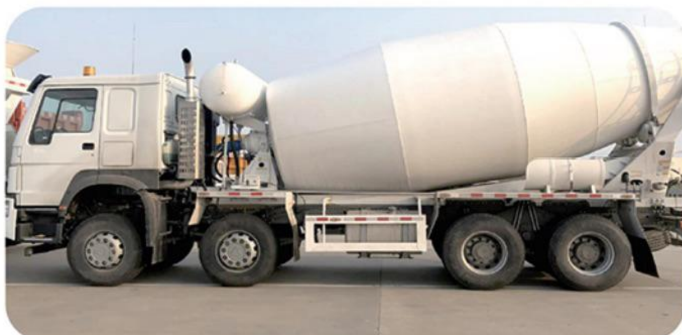
• 12m 3 Mixing Truck •
