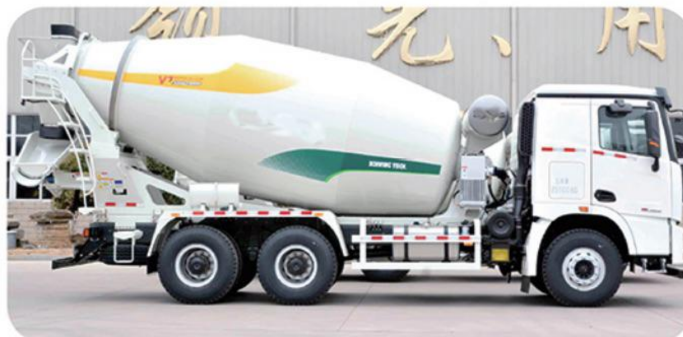
• 8-10 m 3 Mixing Truck •
